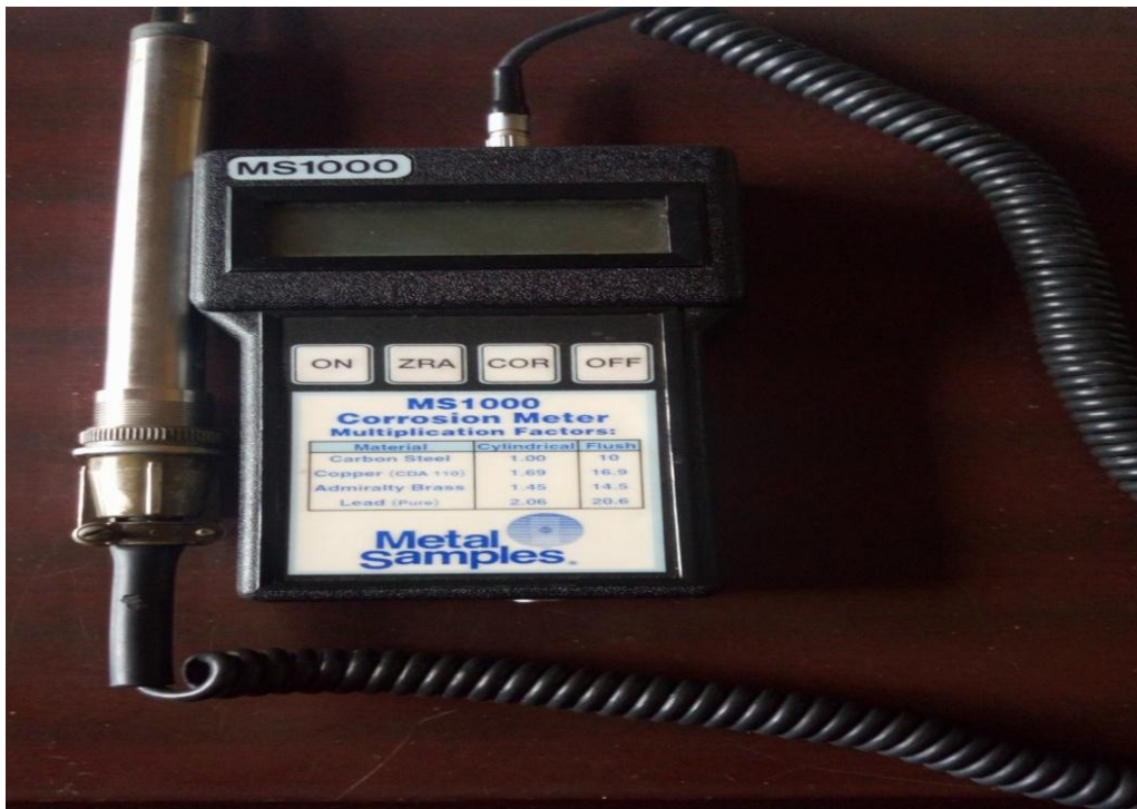
Plate 3.2: MS1000 LPR corrosion meter connected with the probe
