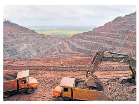
So as per the day to day life bauxite is important for many aspects. The bauxite is then mined using excavators or loaders to load the bauxite onto haul trucks and transported to the crusher.
