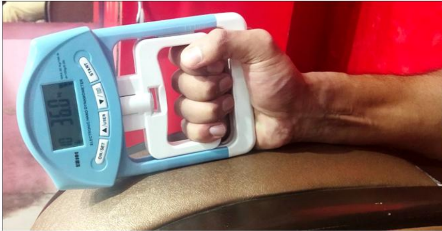
Fig no. 2 Photograph Showing the Measurement of Handgrip Strength by the help of Digital Hand Dynamometer
