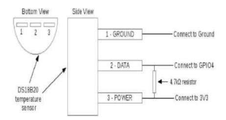
Fig.1 Block diagram of temperature sensor
