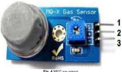
Fig. 4 MQ2 gas sensor
