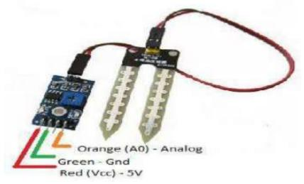
Fig. 2 Soil sensor
