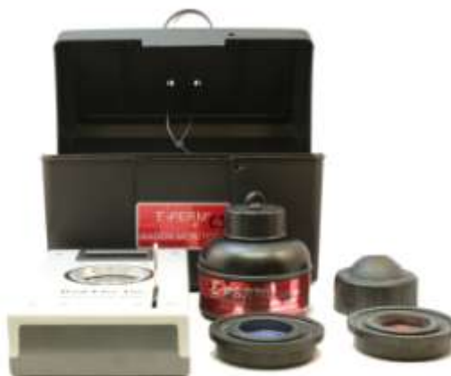
Figure 3. Image showing the equipment used during the study. The elements that compose it are the meter, a tamper-resistant case, a short-time camera, a long-time camera, a short (blue) and a long (red) electret.
