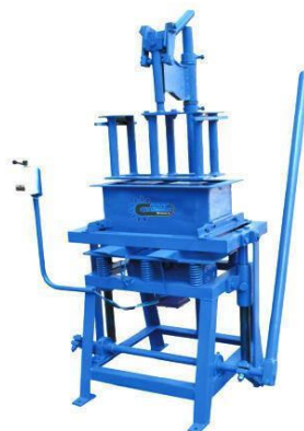
Figure 3: Sandcrete block production machine
