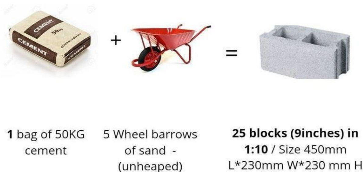
Figure 1: Mixing ratio of sand and cement using wheel barrow
