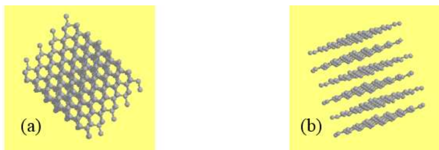
Figure 1.(a) Diamond structure and (b) graphite's layered structure [12].
