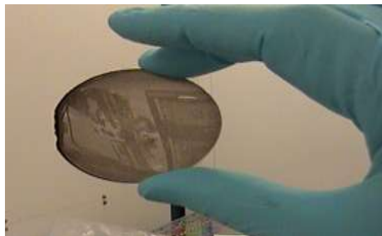
Figure 2. Free standing polycrystalline diamond, ~50 mm diameter and ~230 \mu\text{m} thick.
